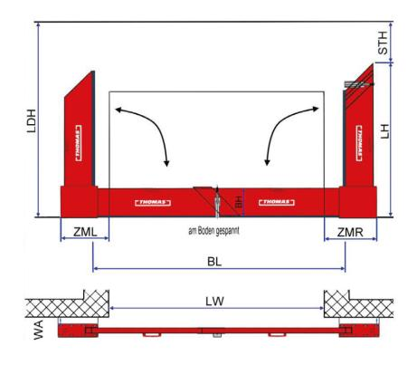
LW - clear openingLH - required heightBH - barrier heightBL - barrier length
