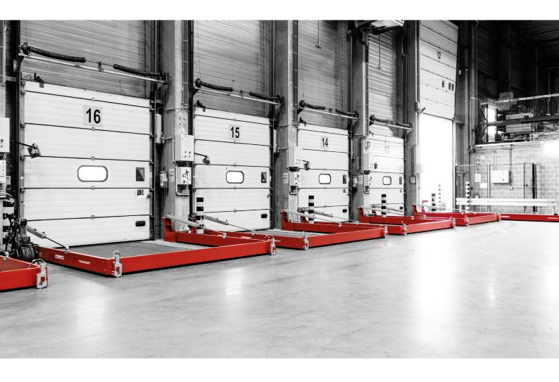
This TÜV and VdS-certified automatic barrier is designed in a U-shape, making it ideal for use at loading docks. The barrier is positioned at rest beside and above the gate opening. The barrier body is held in a vertical position by two pneumatic cylinders.
